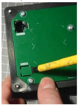
2. Connect the remote equipment to the RJ11 6P4C port using a double insulated data cable (e.g. Clipsal 5005C305B). The pinout for the RS485 cable is shown below:
