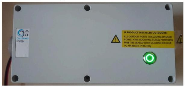
17. When correct operation of the device has been confirmed, insert the plastic screw caps into the 6 lid screw positions:
